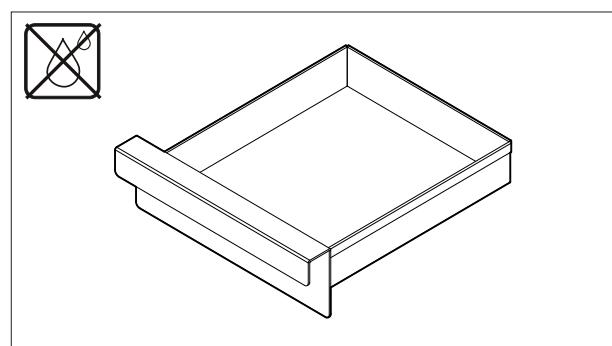
Make the remaining ashes fall into the ash drawers with the help of the poker. Open and close the lower vent repeatedly helping the ash evacuation.
